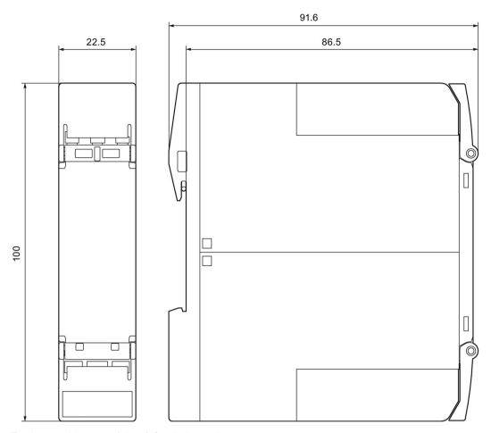
Enclosure 22.5 mm (short) for timing relay:
