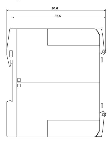
Enclosure 17.5 mm for timing relay:
