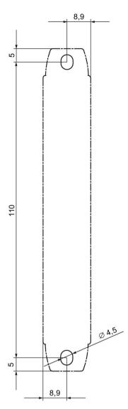
Drilling diagram, enclosure 17.5 mm
