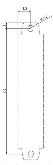
Drilling diagram, enclosure 22.5 mm
