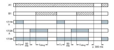
Control signal B1 is open when supply voltage A1 is applied.
