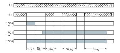
Start contact B1 opens while delta time is running and is applied again.
